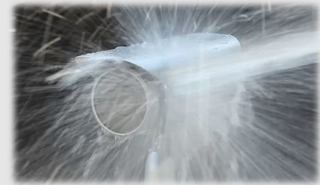
WATERPROOF TEST – IP66
